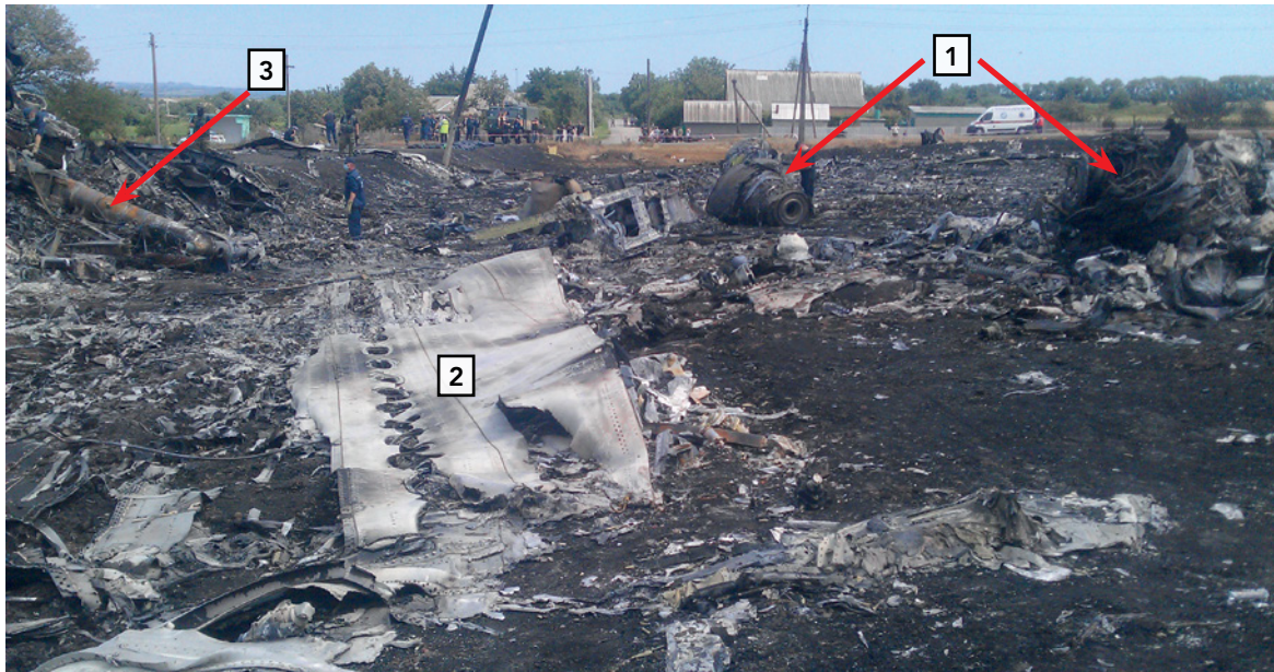
Figure 11: Main wreckage site showing engine parts (1), wing with inspection hatches (2) and main landing gear (3). (Source: NBAAI)
